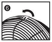
Place the **Front Safety Grille** into position and secure it by closing the clips over the outer rim.
