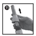
Loosen the **Height Adjustable Locking Ring** and extend the support pole to your desired height.
