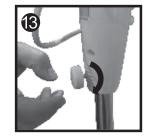
Take the fan assembly and place it onto the pole and tighten the **Pole Screw** by hand.
