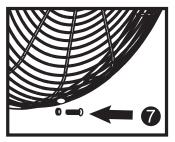
Using the **Small Nut and Bolt**, fasten the two grilles together.
