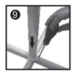
Fix the **Pole** on the cross base and refit the 4 fasteners and tighten.
