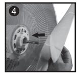
Place the **Fan Blade** onto the motor spindle.
