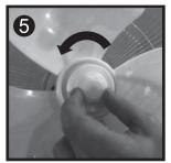
Fix the blade into place by gently hand tightening the **Spinner Nut** (anticlockwise) onto the end of the motor spindle.
