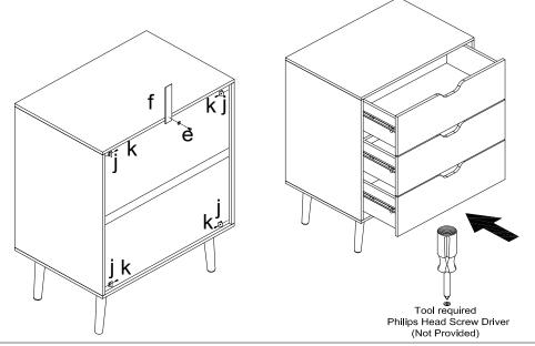
**Step 6:** Fix screw a onto board (7), and put part b & c into the corresponding position (as per below diagram). Then fix board (8), (9), (11) to board (7) by tightening part b. Slide board (12) into the corresponding position, fix board (10) with screw i.
