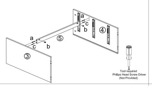
**Step 2:** Slide board into the corresponding position (as per below diagram). Ensure it is fully fitted in the groove.
