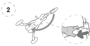
Locate the circular lever on the underside of the ScuttleBug^TM, pull back (in the direction of the arrow) to unlock and release the front wheel stem.
