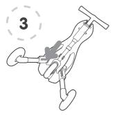
Fold the front wheel strut down into the underbody. Pull the wheel to extend and slot into the clasp.
