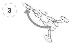
Hold the front wheel and pull out to release from the plastic clasp. Pull forward (in the direction of the arrow) until it locks into place.
