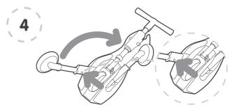
Fold the rear wheel by using your finger to press down the spring loaded button on the inside of the sleeve. Once fully compressed, maintain pressure on the button and slide the sleeve outwards (in the direction of the arrow shown on the rear of the sleeve) to release it from the locked position. Fold inwards (in direction of the arrow shown in the diagram) until the rear leg locks into place. Repeat for the other rear wheel.
