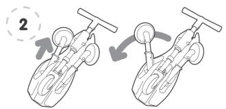
Unfold the rear wheel by pulling rear sleeve towards the wheel (shown by the arrow on the sleeve) to release it from the locked position. Pull outwards (in the direction of the arrow on image) until it locks into place. Repeat for the other rear wheel.
