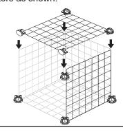
STEP 4. Insert three grid panels (A) into slots.
