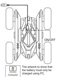
Charging time: approximately 90 mins (the light is red, that means charging now. The light is off, that means the battery is full).
