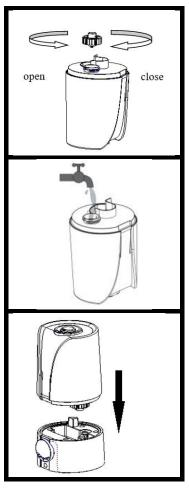
2. Turn the tank upside down and remove the tank cap by turning it counter-clockwise
