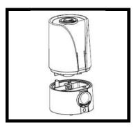
1. Remove the mist nozzle and Lift up water tank from humidifier base
