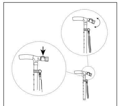
To turn on the LED light, press the on/off button one time.
