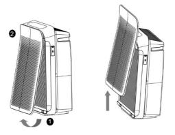
**IMPORTANT!** Check that the air inlet grille is properly hooked on to the main unit and bottom interlocks are fitted properly, or the unit will not turn ON.
