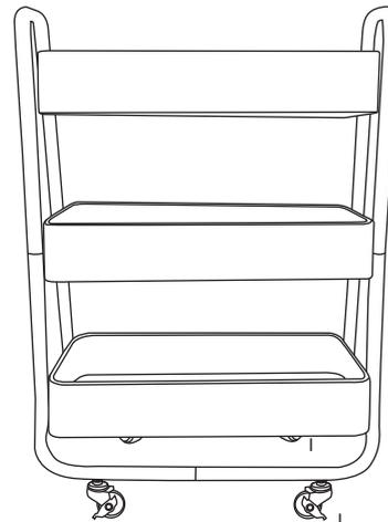
5. Assemble the wheels (i)(j) to the bottom. Use the spanner (h) to tighten.
