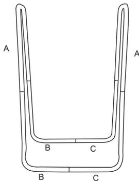
2. Connect the top tube (a) to the tubes (b) and (c).
