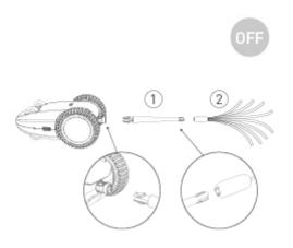
2. Insert the charging cable into a power charger adapter and into the mouse. Charge the device until the power indicator (red light) turns off. Ensure that the device is switched off before charging.
