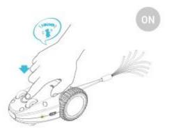
4. Pat the device and put it on the floor, and it will move in auto mode. Pat it to reactive the mouse in the standby mode.
