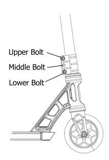
1. Loosen the clamp on steering tube. Slide the tube onto the fork until it is touching the fork headset washers.
