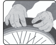
FIGURE A Press with thumbs to separate tyre bead. Continue around entire rim until the bead is completely separated.
