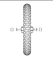
Insert the bearing Nut from B into both sides of Rear Wheel. The White plastic spacer is to be placed between the wheel and frame.
