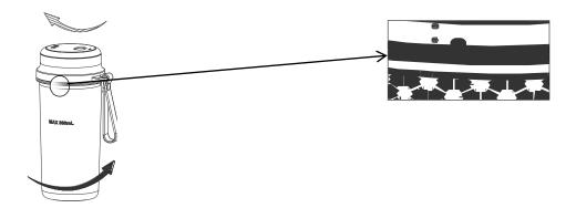
4. Double-click the button switch on the main unit, turn the blender upside down, put it on a tabletop or hold it in your hand, and the blender starts to operate. **The blender has a single operation time of 40 seconds.** When the blender is operating, it can be shaken from side to side to improve the blending process.
