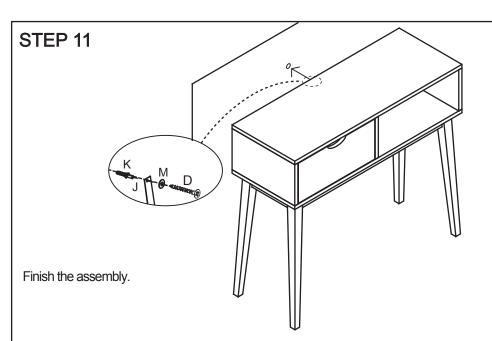
Predrill the hole at wall, insert part K into hole, attach Anti Tip Strap J with part D & M into the corresponding position as per diagram.
