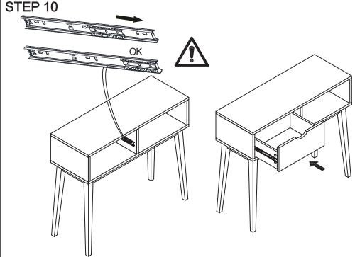
Attach the drawer onto Step 6 and then adjust drawer runner into corresponding position as per diagram.
