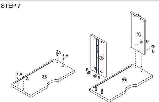
Fix part A onto board 11 into the corresponding position as per diagram. Attach board 7 & 9 onto board 11 with part B.
