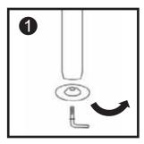
Unscrew the Locking Lever and washer from the bottom of the stand post.
