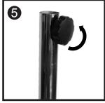
Unscrew (anticlockwise) and remove the Locking Knob from the top of the stand upper post.
