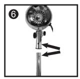
Sit Motor Housing on top of Stand Post with the hole in the neck and the hole on the upper post aligned as shown.
