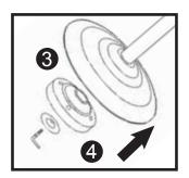
Tip up the Base and place the Weight in the centre of the base. Fasten in place by use of the Locking Lever and washer and tighten.
