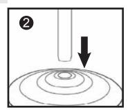
Insert the bottom of the Stand Post through the hold in the top of the Base.
