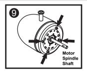
Remove the protective plastic sleeve from the motor spindle shaft and the 4 screws as Identified.
