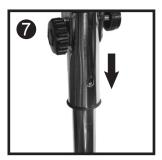
Push the head down onto the upper post until the two holes are overlapping.
