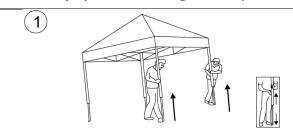
Remove any leg stake and guy ropes, You and your partner should each lift up two adjacent outer legs slightly, depress the snap button and push the telescopic inner legs into the outer legs. Repeat for the remaining two legs.
