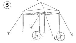
Use the guy ropes attached to the ring at each corner of the roof cover and stakes, to secure your fold up Gazebo to the ground or just use the stakes through the holes in each legs foot.
