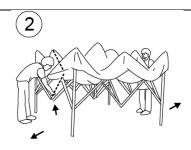
Put the canopy on it. Each partner should grasp the top and bottom of the diamond formed by the side supports on opposite sides and pull hands together while stepping backwards until the shelter is fully opened. Be careful not to pinch your fingers or to pull backwards too hard as this will result in the side supports bending.
