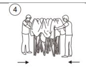
Grasp the two outer legs, slightly lift off the ground and push together to fully close.
