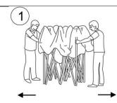
Place your fold up Gazebo in the center of the area to be sheltered. Remove the carry bag and stand the fold up Gazebo on its' feet. With partner on the opposite side, grasp two outer legs, slightly lift the frame off the ground and take a step backwards, stepping at full (outstretched) arms length.
