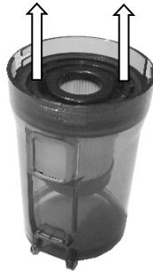
Grasp the outer filter body and with the other hand, grasp the tabs of the inner filter and rotate anticlockwise to unlock, then pull up and out.
