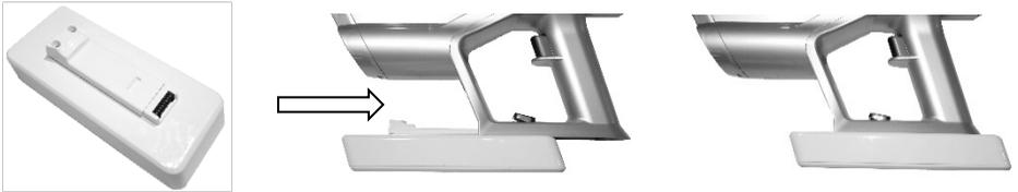
To Remove the battery, press the release button located inside the handle area, and at the same time, pull the battery straight out.
