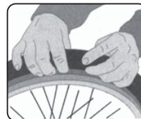
FIGURE A Press with thumbs to separate tyre bead. Continue around entire rim until the bead is completely separated.
