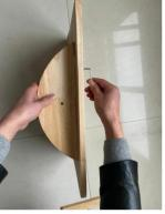
Align the semicircle board to the main board, then take the screws and pass through the hole, use the hex wrench to tighten
