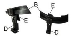
Step 4. Connect the two parts of step 2 & 3 together at three positions, then secure them with screws (Part B1).
