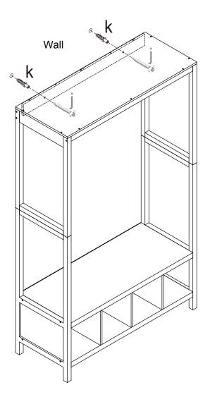
It is strongly recommended that this product is permanently fixed to the wall. Please seek professional advice if you are in doubt of what fixing device to use. Regularly check that anchors are securely maintained.
