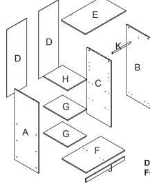
Do not tighten the screws fully during assembly. Fully tighten screws after the final assembly steps
