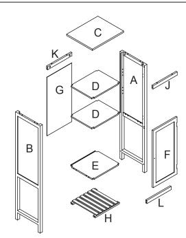
Do not tighten the screws fully during assembly. Fully tighten screws after the final assembly steps
