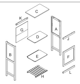
Do not tighten the screws fully during assembly. Fully tighten screws after the final assembly steps
