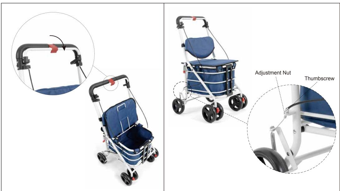
1) When you want to use the brake, pull on the brake rod, this can be locked in place by using Lock A. Make sure that you lock the brake when you want to sit on the seat. Use the lock when you are loading the basket or if you want to remain stationary. 2) Hold the thumbscrew firmly in place, do not turn.To tighten the brake, turn the adjustment nut counter-clockwise;To loosen the brake, turn the adjustment nut clockwise.
