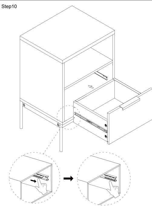
Slide ball bearing slide part to top of rail when assembling the drawer.
