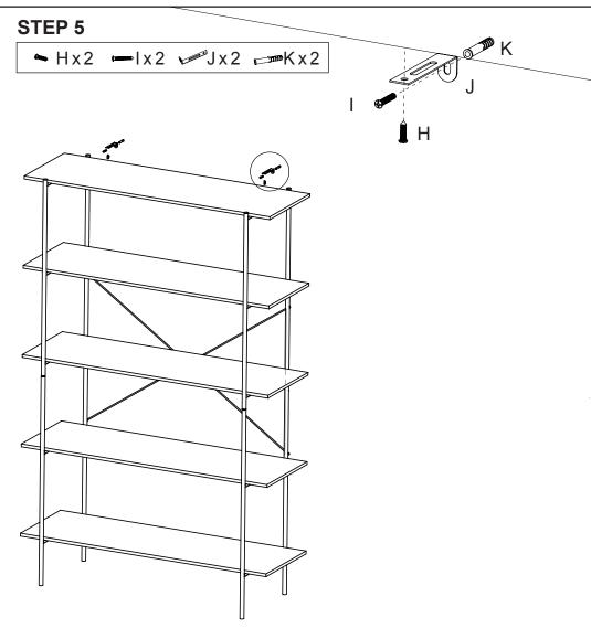
It is strongly recommended that this product is permanently fixed to the wall. Please seek professional advice if you are in doubt of what fixing device to use. Regularly check that anchors are securely maintained. **CAUTION:** for your safety when attaching the anchor fixings, please note the following: Check any electrical wires or plumbing inside the wall before drilling any holes
