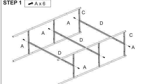
ATTENTION: DO NOT TIGHTEN THE SCREWS FULLY DURING ASSEMBLY.FULLY TIGHTEN SCREWS AFTER THE FINAL ASSEMBLY STEP.
