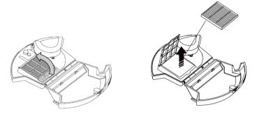
Grasp the tag on the white filter and pull up and out
