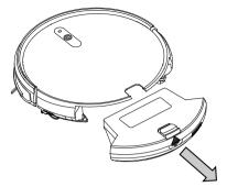
• Pry open the dust canister lid and swing open, then empty into the bin.
