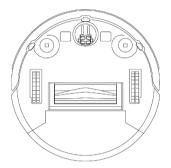
Position the side brushes, with the square holes pointed down, and the brush bristles angled up. Align the square hole, on the underside of the side brush, over the square post, located inside the hollow circle. Push down hard until it clicks in place. It does not matter which brush goes on which side.
