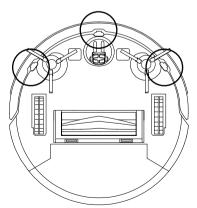
Keep these sensors clean by wiping with a dry cloth or brush them using the cleaning brush supplied.
