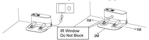
**NOTE**: If the IR signal emission window is blocked, the robot will be unable to locate the charging dock.
