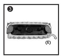
Lift the outer edges of the clamps of the holder and peel the **Large Microfibre Pad(E)** off from the corners. Simply wash and dry the mop pads.
