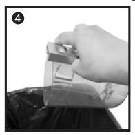
Empty the **Dust Canister** into a rubbish bin and remove any debris from the filter and filter holder by tapping on the edge of the rubbish bin.
