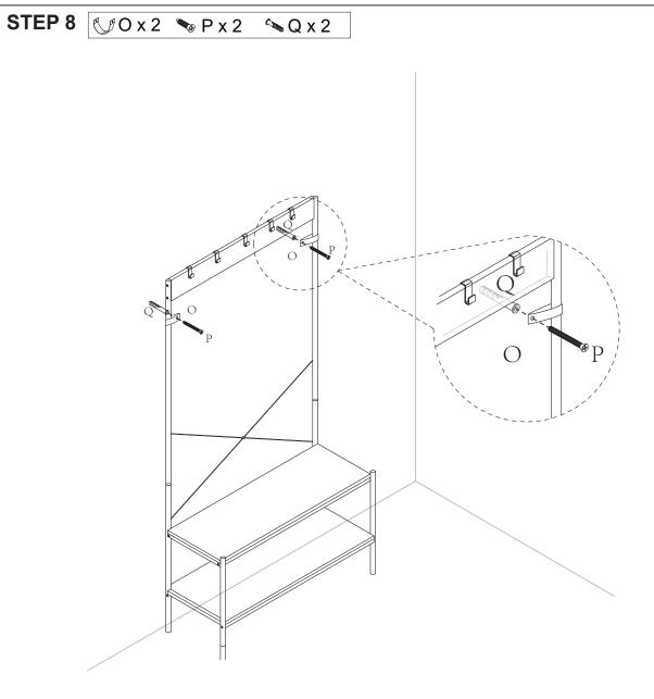
It is strongly recommended that this product is permanently fixed to the wall. Please seek professional advice if you are in doubt of what fixing device to use. Regularly check that anchors are securely maintained.
