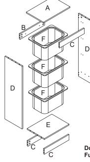
Do not tighten the screws fully during assembly. Fully tighten screws after the final assembly steps
