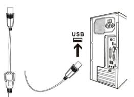
Insert it into the USB ports of the computer. If you use a desktop computer, it is best to plug it into the USB ports on the back of the computer case instead of the USB ports on the front.
