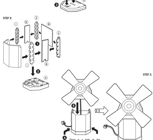
There is a hole at the bottom of each side for the wire
