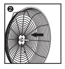
Fit the Back Safety Grille into position and refit the 4 Screws and tighten. (\*Note: The handle on the back of the grille should be at the top)
