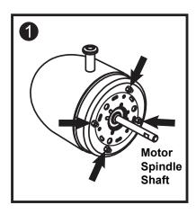
Remove the protective plastic sleeve from the motor spindle shaft and the 4 Screws as identified
