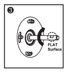
Rotate the motor spindle until the "FLAT" surface is facing up.
