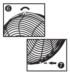
Place the Front Safety Grille into position and secure it by closing the clips over the outer rim.
