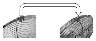
Secure the grille by closing the clips over the outer rim.
