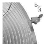
Place the safety grille into position by lining up the slot in the location plate over the top of the rear grill and over the wire spoke as shown and push down.
