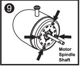
Remove the protective plastic sleeve from the motor spindle shaft and the 4 screws as Identified.
