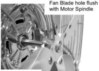
**Tighten Fan** Blade Screw
