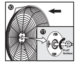
Slide and push the **Fan Blade** onto the spindle. Push on until the end of the fan blade hole is aligned with the end of the spindle.
