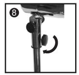
Screw in the **Locking Knob** (Clockwise) and nip up. Do Not overtighten.
