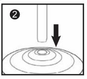
Insert the bottom of the **Stand Post** through the hold in the top of the **Base**.
