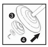
Tip up the Base and place the **Weight** in the centre of the base. Fasten in place by use of the Locking Lever and washer and tighten.
