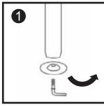
Unscrew the **Locking Lever** and washer from the bottom of the stand post.
