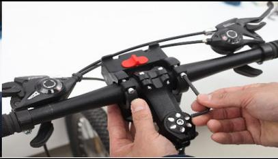
3,Tighten the bottom support screw
