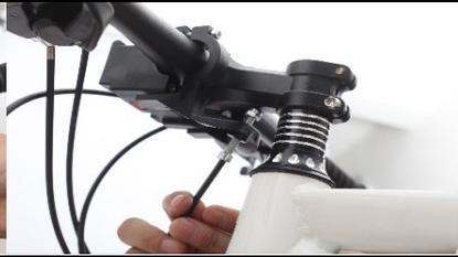
4,Install the basket onto the mounting slot
