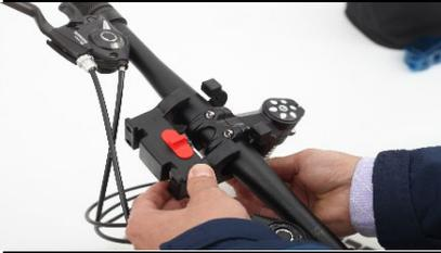
2,Tighten the four screws to fix the buckle
