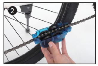
2. Slide the handle off, push the top cover and lift it to open, insert the chain into grooves.
