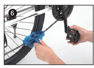
Hold the chain cleaner with your hand whilst using another hand to spin the pedal backwards a few times until you satisfied with the chain cleanliness.
