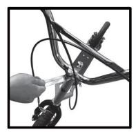
Step 1. Insert the stem pillar into the fork tube to the minimum insertion line, indicated on the stem pillar. Face the handlebar stem forward directly in line with the front wheel. Tighten the stem pillar bolt to a torque requirement of 15-17N.m
