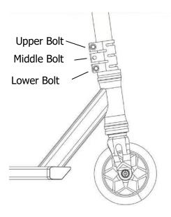
1. Loosen the clamp on steering tube. Slide the tube onto the fork until it is touching the fork headset washers.
