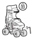
2. Separate the boot and the chassis.
