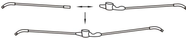
Step 2. Assemble the loop of bowstring (Part C) to one end of the bow around the groove, then make the bow stand vertically (reference image). Press the upper side of the bow to ensure the other loop of bowstring is assembled into the bow.
