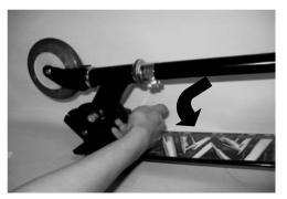
Step 3: Release the scooter handle by pressing the bullet.
