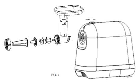
**Note:** Never assemble blade and cutter when making sausages, and do not assemble the sausage pole and kibble cone when mincing meat.
