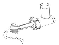
4. Press the rocker switch to "ON" position. The appliance will turn ON and the minced meat will enter the sausage casing. Tie anywhere you like with thread to make the sausage.
