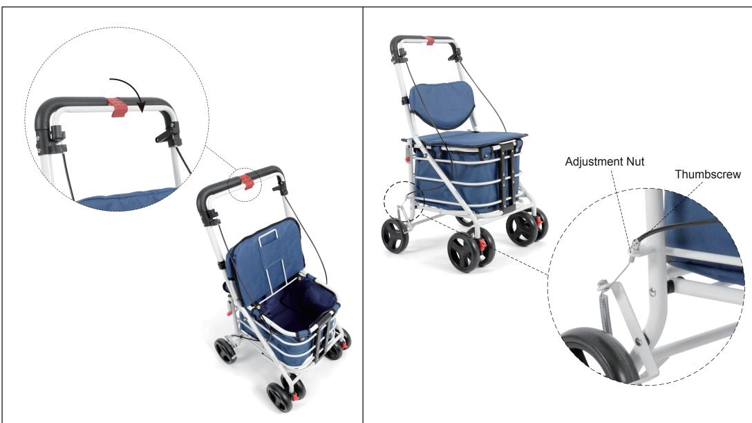
1) When you want to use the brake, pull on the brake rod, this can be locked in place by using Lock A. Make sure that you lock the brake when you want to sit on the seat. Use the lock when you are loading the basket or if you want to remain stationary. 2) Hold the thumbscrew firmly in place, do not turn. To tighten the brake, turn the adjustment nut counter-clockwise; To loosen the brake, turn the adjustment nut clockwise.
