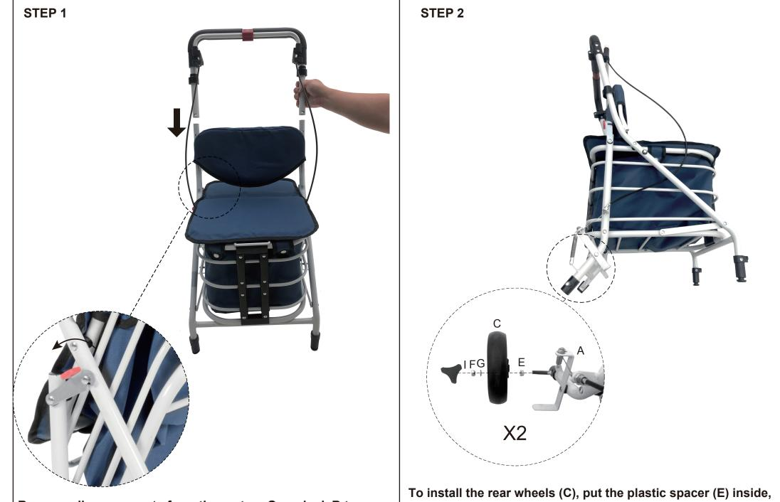
Remove all components from the carton. Open lock B to release the trolley and insert handle bar into the handrail tube.
