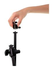
Mount the ball head to the Tripod stand with 1/4 inch mounting screw, tightened screw cap after the connection;
