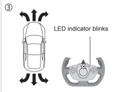
When LED indicator goes out, pairing process is completed.
