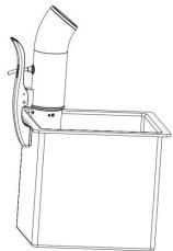
Firmly lock the appliance by clamping it on the side of the container. Make sure the clamping surface is completely in contact with the wall of container.
