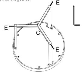
Step 2: Use screws (Part D) to fasten metal legs (Part B) to the board (Part A).
